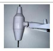
3. There is a fixing screw between the wind speed and wind direction sensors. Loosen this screw.
