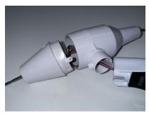
5. Unplug the two 5-pin connectors and remove the them from the wind speed and direction sensor unit.
